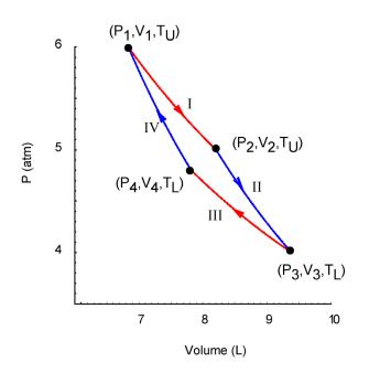
$P_1$ = 6 atm,  $T_1$ = $T_U$ =500K  $P_2$ = 5 atm,  $T_2$ = $T_U$ = 500K  $q_{II}$ =0  $P_3$ =4 atm,  $T_3$ = $T_L$
