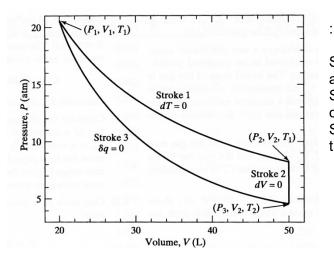
Stroke 1 is an isothermal expansion at  $T_1$ . Stroke 2 is a constant-volume
