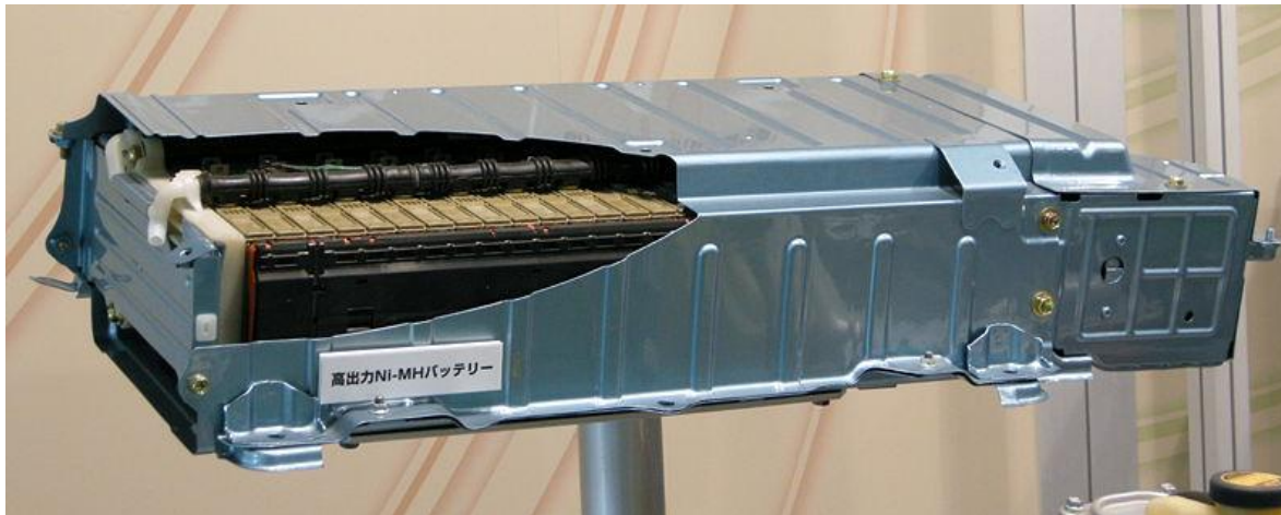
High power Ni-MH battery of Toyota NHW20 Prius
