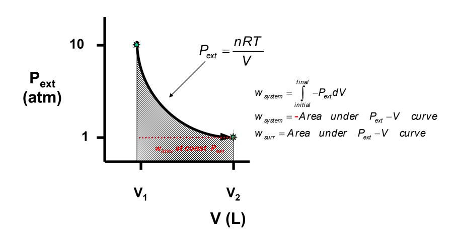
Pressure-Volume work reversible isothermal expansion; P<sub>ext</sub>=P<sub>int</sub>
