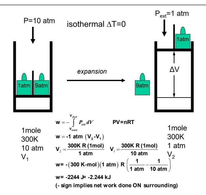
Pressure-Volume work reversible isothermal expansion; P<sub>ext</sub>=P<sub>int</sub>
